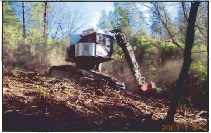
Large masticator works on slopes up to 40% and reduces unwanted vegetation from 20 feet high down to ground level mulch. Here a rotary head “chews up” the vegetation.
